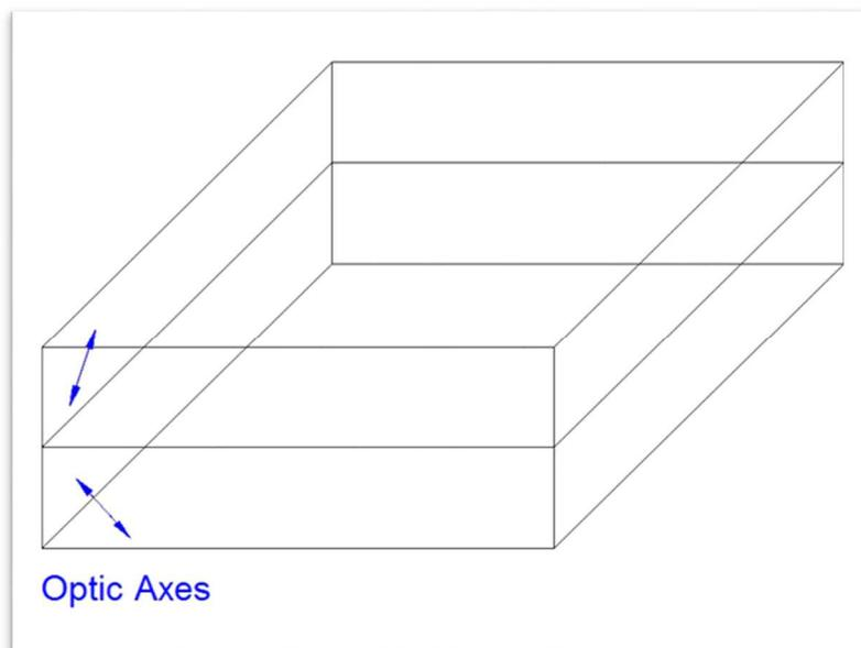
The beam displacement produced by the savart plate is approximately 0.075 times the total thickness in calcite and 0.0042 times in quartz. When ordering a Savart plate we need to know the material, aperture and thickness required, as well as if AR coatings and a mount are required.
